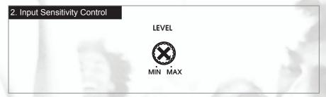
This control adjusts the amplifier's input sensitivity. The input sensitivity is variable from 200 Millivolts to 8 volts. Turning clockwise increases sensitivity. Turning counter clockwise decreases sensitivity. **This knob is not a volume control for the amplifier**. The amplifier can be driven to full power with a wide range of input signals. A lower signal level will require increased sensitivity to reach full power. A higher signal level will require decreased sensitivity.
